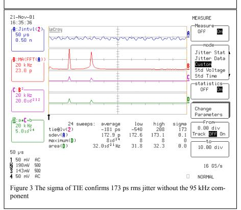
yields173 ps rms jitter from spectral components in the range of 0 to 77 kHz. Figure 3 shows a confirmation of this value based on removing the 95 kHz
