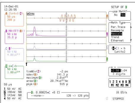
Figure 1– The mean squared (Area) and rms( sdev) jitter of a 400 MHz carrier modulated by a 50 KHz sine burst with a duty cycle of 20%.
